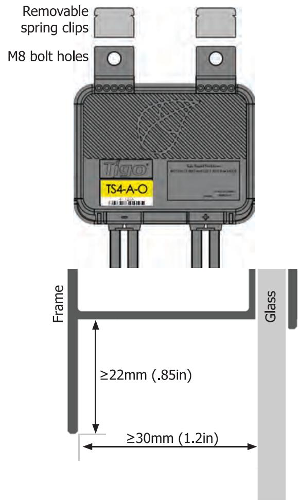
The distance between an attached TS4 and module substrate must be  $\geq 12.7\text{mm} (.5\text{in})$ .
